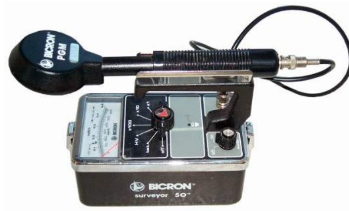
Radiation survey meter onsite: Surveyor 50 Portable GM
