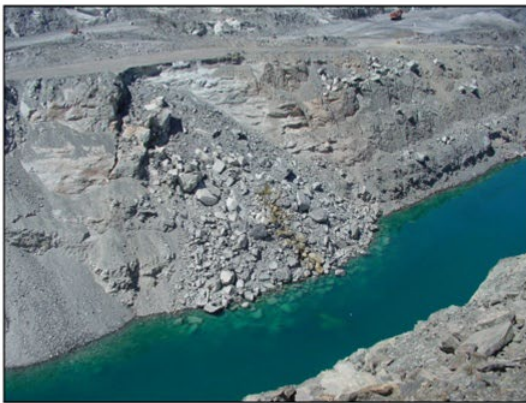
Slope failure impacting haul ramp
