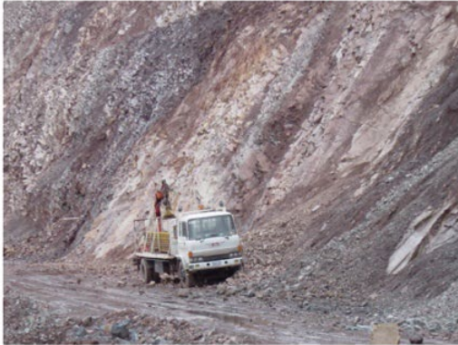
Flatbed truck parked inappropriately. Vehicles should not be parked near slopes. If this can not be avoided, vehicles should be reverse parked.
