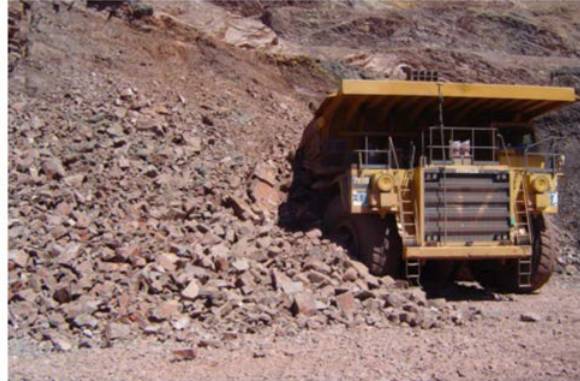
Slope failure impacting haulage truck.
