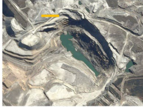
Mina Pecket Mine slope failure resulting in cessation of mining (yellow bar is 200m long for scale)
