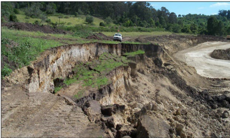
Example of a circular failure in weak soil.
