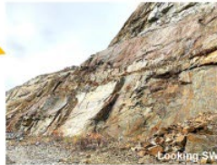
Major discontinuities on the footwall, guiding the historical slope angles.
