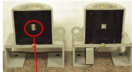
Cutaway of a source holder
