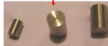
Double sealed metallic capsules containing radioisotope
