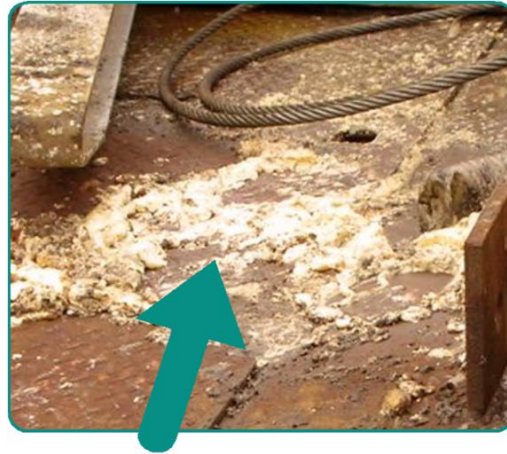
Emulsion type explosive on the deck of a scissor truck
