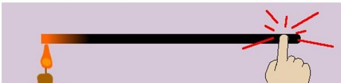
Flame heats the metal rod, metal rod conducts the heat to the end of the rod.
